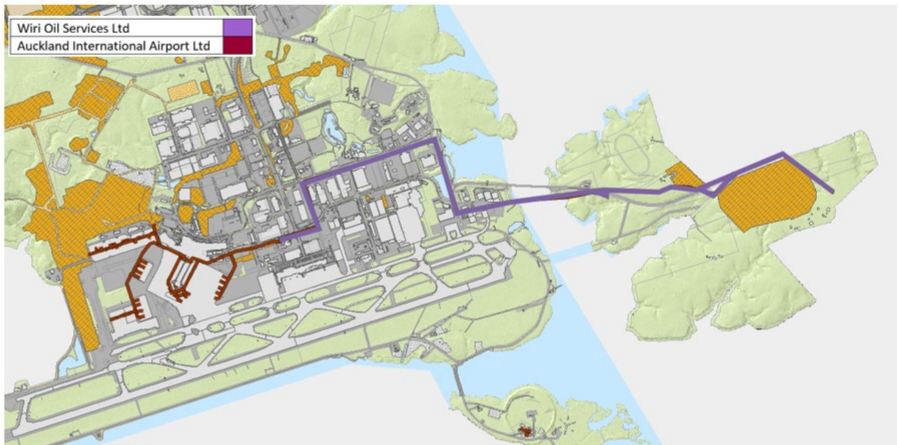
Fuel Pipeline and Fuel Hydrant System
