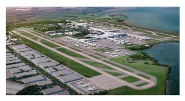
An OLS extends outwards from a runway centre line restricting the maximum height of obstacles such as buildings and trees in the airspace surrounding the airport. This means that aircraft can safely manoeuvre at a low altitude.
