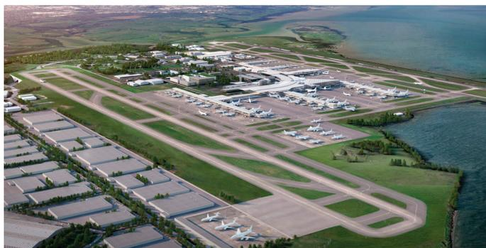
An OLS extends outwards from a runway centre line restricting the maximum height of obstacles such as buildings and trees in the airspace surrounding the airport. This means that aircraft can safely manoeuvre at a low altitude.
